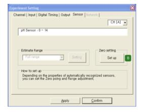
3. Confirm pH figure while sensor is still soaked in KCl solution as shown below in 1 of image. (The figure should show approximately 3.9 if in safekeeping solution)
