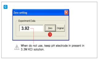
4. Calibrate electrode in pH 7.0 standard solution and pH 4.0 standard solution as shown below in 2, 3 of image.
