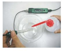
• When the probe is not being stored in the storage bottle, it can be stored
