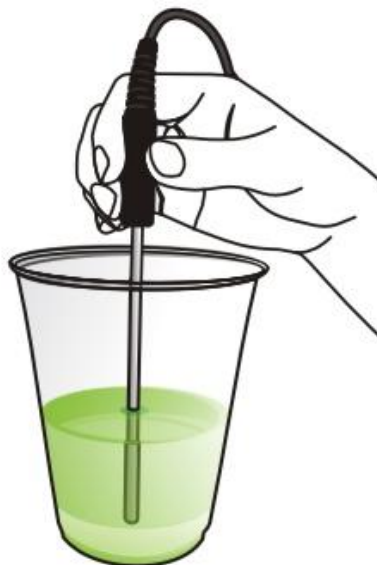
Fig.1 An easy experiment with everyday materials like water, soda and water cup. In this activity, you can plot the temperature graph of the liquids with cooling time.
