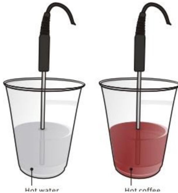
Fig.4 Measure the temperature of a cooling water and coffee and inquire how hot coffee get cool enough. In this experiment you can gather simultaneously from two temperature sensors, and while the data are being collected, you can construct a mathematical model of the experiment and determine whether the exponential model fits the data as like the formula shown below.
