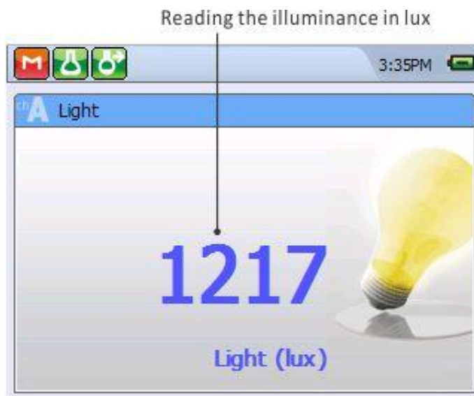
Fig.2 Reading the illuminance in lux. While you are reading the illuminance in lux, you can take the values which will vary depending on the direction of the light source and the lighting environment.
