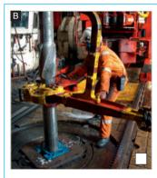
I work on an offshore oil rig. I spend a lot of my time tripping drill pipe in and out of the hole, and operating the tongs to make or break connections. I also do other jobs around the rig, such as looking after equipment.
