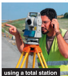
using a total station
